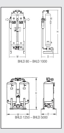
The all-in one package for dry compressed air: The ideal solution for compressed air pressure dew points below 38°F. The heatless BOGE adsorption dryers can reach dew points of -70°F (standard -40°F). The twin tower system allows regeneration simultaneously with the adsorption eliminating the need for any external power supply.
